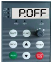
Fig 3-1 Power-on Parameter Display Initialization Display "P.OFF"
