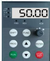
Fig 3-2 Stop Status Parameter Display Display Set Frequency "50.00"
